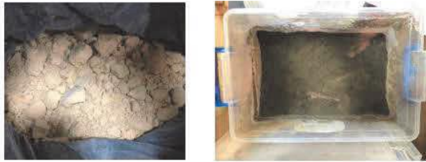
Figure 1. Natural (left side) and burned (right side) filter sludge
