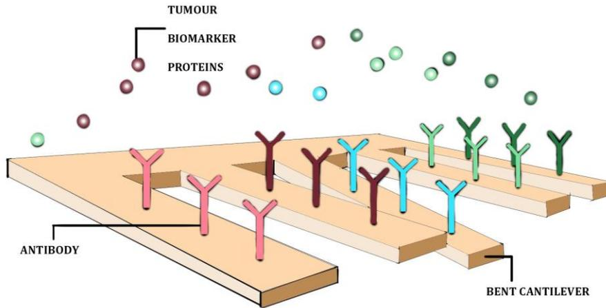
Fig 7. Nano-Cantilever working mechanism [133]. Reprinted by permission from Elsevier.
