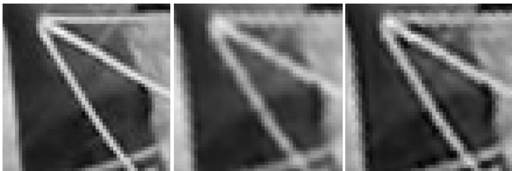
Figure 6. A magnified edge region in a) downsampled original. b) SR with "iterative norm 2". c) SR with proposed algorithm (IBP with edge preservation).
