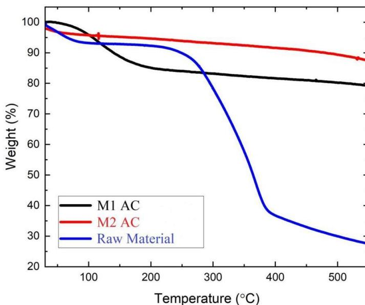
**Fig. 3** TGA data of the raw sample, M1, and M2 samples.
