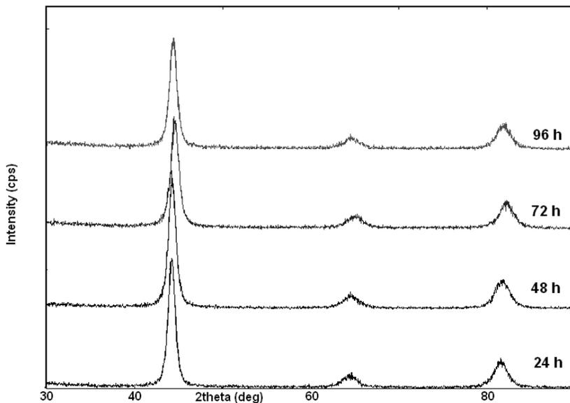
**Fig. 3.** X-ray diffraction patterns of Fe<sub>80</sub>Al<sub>20</sub> alloys after different mechanical alloying times.
