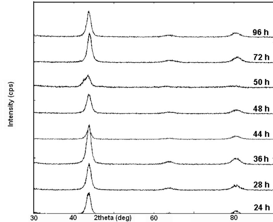
**Fig. 4.** X-ray diffraction patterns of  $\text{Fe}_{50}\text{Al}_{50}$  alloys after different mechanical alloying times.
