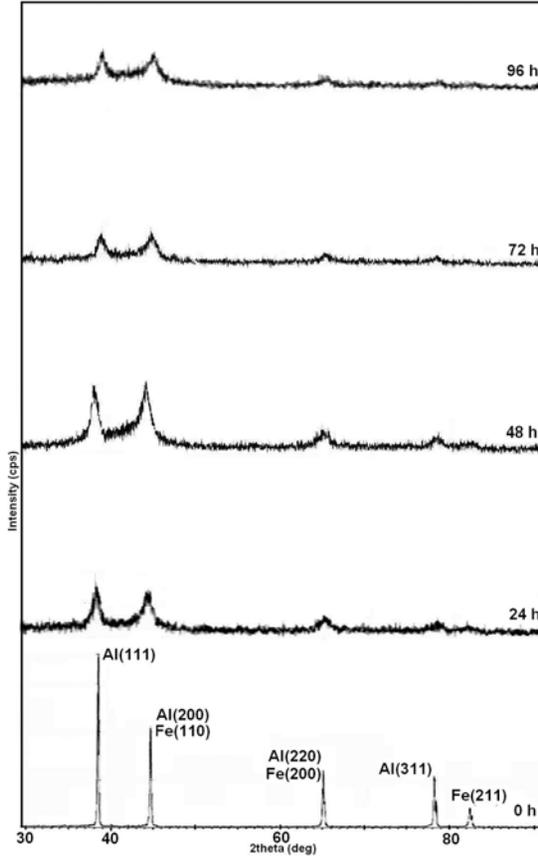
**Fig. 2.** X-ray diffraction patterns of Fe<sub>10.8</sub>Al<sub>89.2</sub> alloys after different mechanical alloying times.
