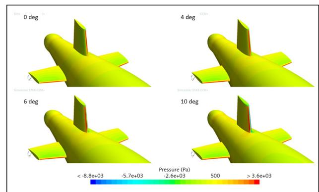
Figure 16. Pressure Distribution on Aft Body of Submarine.
