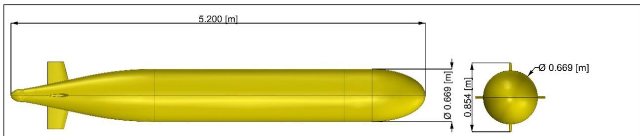
**Figure 3.** Autosub Geometry Top View and Back View.
