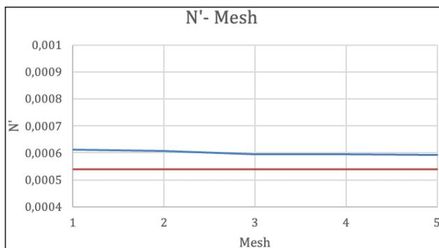
**Figure 8.** Yaw Moment N' for drift angle 6 degrees.
