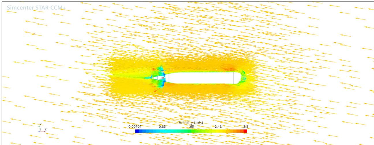
**Figure 17.** Vector Field Around the Submarine.
