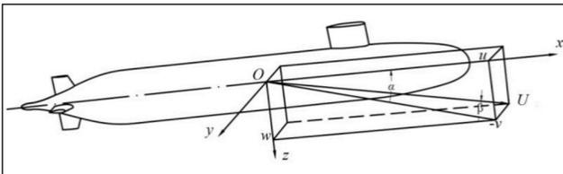
**Figure 1.** The coordinate systems (Zhao et al., 2022).
