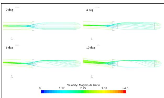
Figure 15. Streamlines Around the Submarine.
