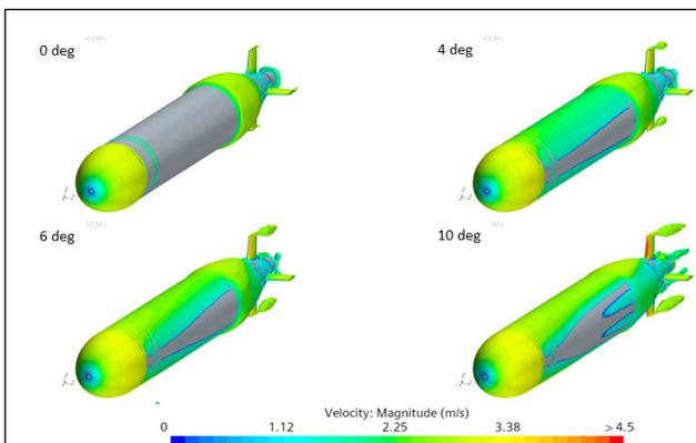
Figure 14. Q Criteria = 5 Surfaces Around the Submarine.
