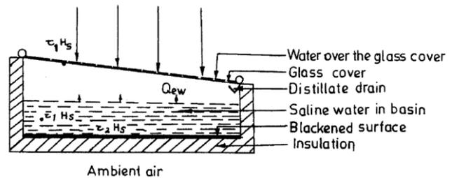
Figure 2. Solar still with water flow on glass [13].
