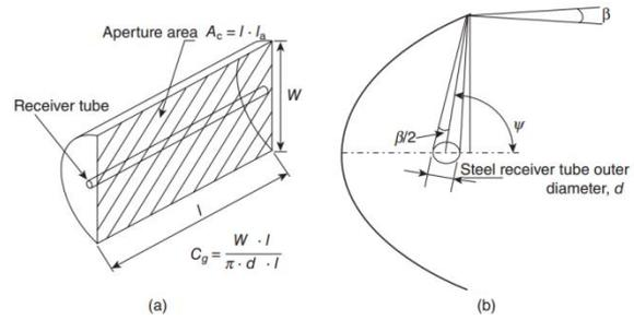
Figure 7. Geometry of the Parabola [45].
