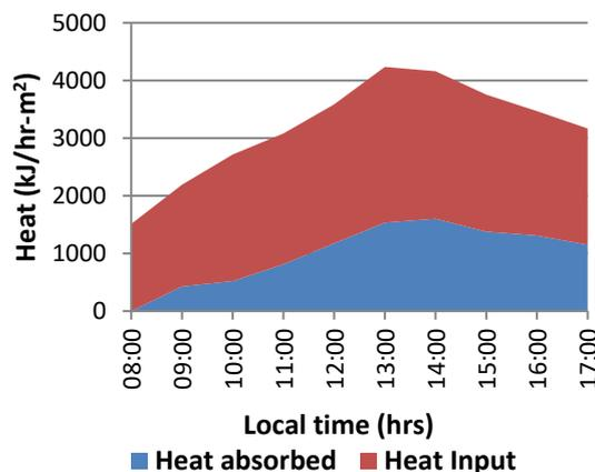
Figure 17. Heat input and absorbed for PTC coupled solar still.
