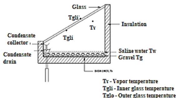
Figure 4. Solar still with internal heat exchanger [18].
