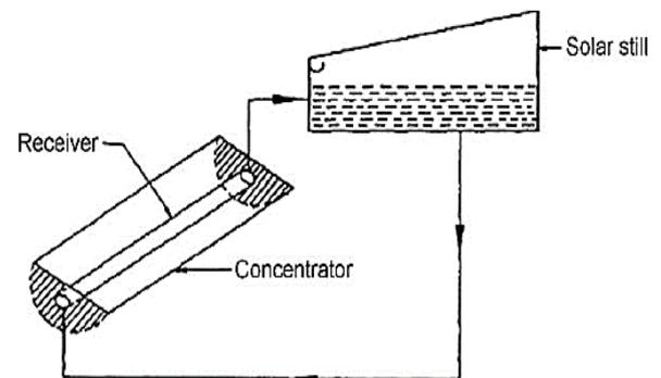
Figure 6. Solar still coupled with parabolic trough collector [29].
