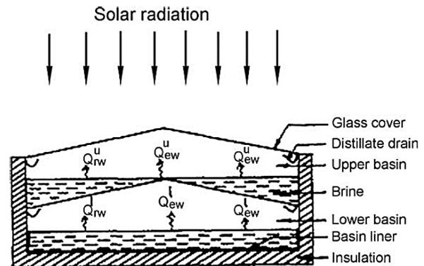
Figure 5. Double slope double basin solar still [23].
