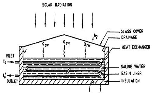
Figure 3. Solar still with internal heat exchanger [16].
