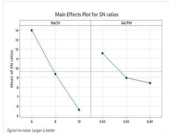
**Figure 5.** S/N ratios flexural strength by parameter levels
