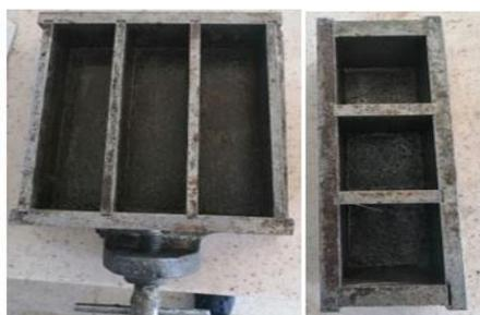
**Figure 2.** Beam and cubic molds used in experiments
