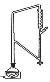
Figure 2. Clevenger apparatus
