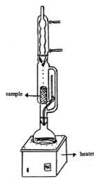
remaining oil is measured. The percentage of oil in the initial sample can then be calculated.
