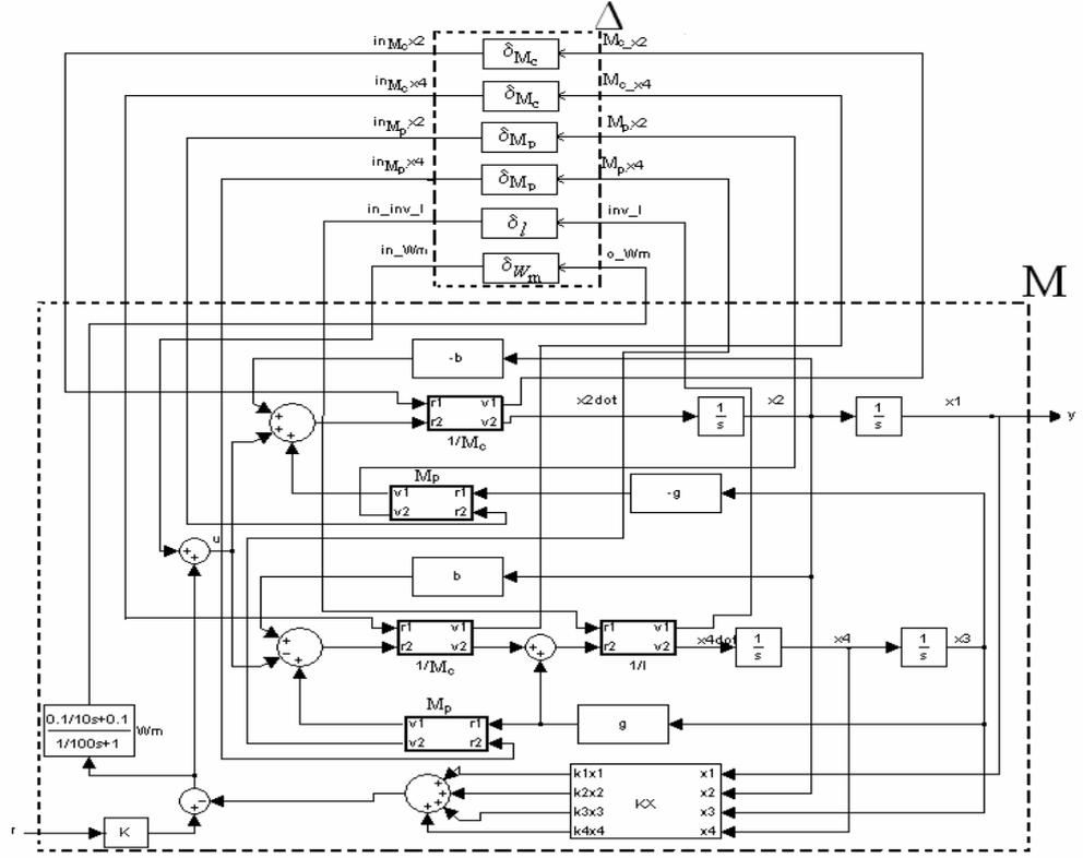
Figure 6. A detailed block diagram of the interconnection  $M$  and  $\Delta$
