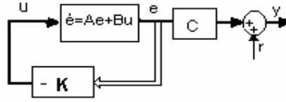
Figure 2: Block diagram of the feedback system with error states
