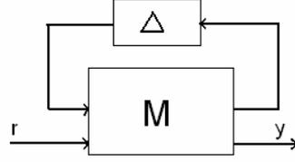
Figure 3. Macro model of inverted pendulum system with uncertainties
