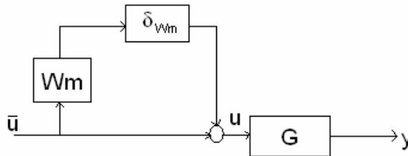
Figure 5.c Unmodeled uncertainty at the system input
