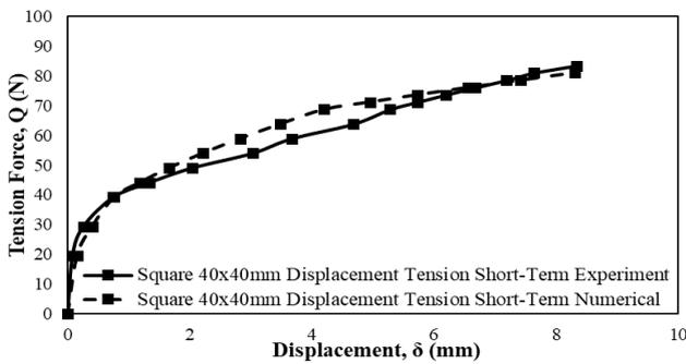
**Figure 10.** Square (40x40mm) displacement piles short-term results
