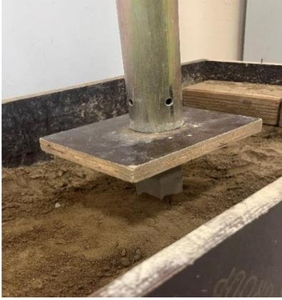
**Figure 4.** Displacement pile application process
