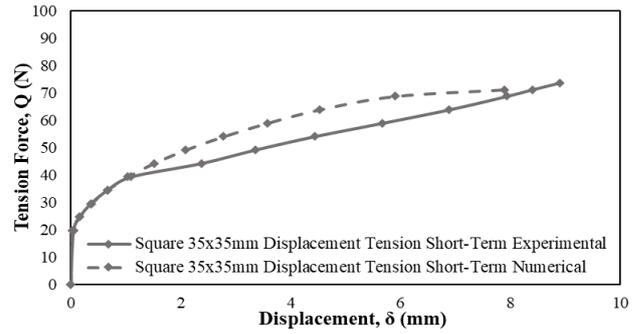
**Figure 11.** Square (35x35mm) displacement piles short-term results
