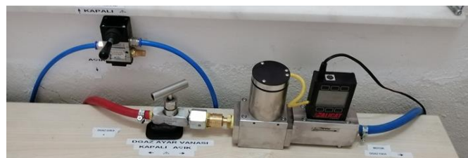
Fig. 4. Natural gas flow control unit
