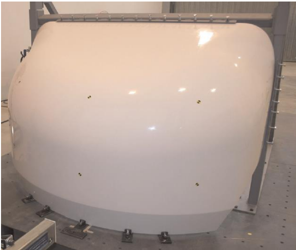
Fig. 12. A prototype of the frontal composite structure [46]
