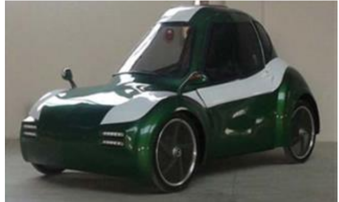
Fig. 7. Fiber-glass body structure of an L7e vehicle; Hu-Go [20]
