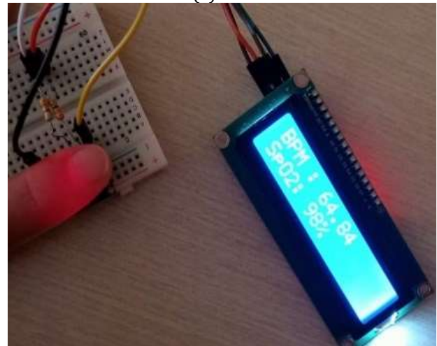
(b) Hearth Rate (Beat Per Minute) and percentage of oxygen in blood (SpO2)
