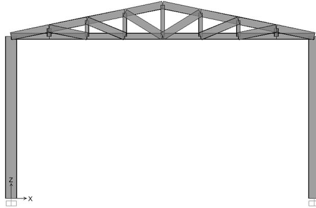
Figure 8. Industrial structure with optimum profiles without corrosion effect
