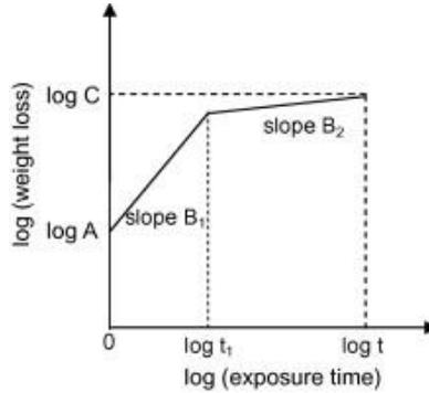
Figure 4. Schematic diagram of the variation of the thickness loss of mild steel in the marine atmosphere with time in log-log coordinate [8]
