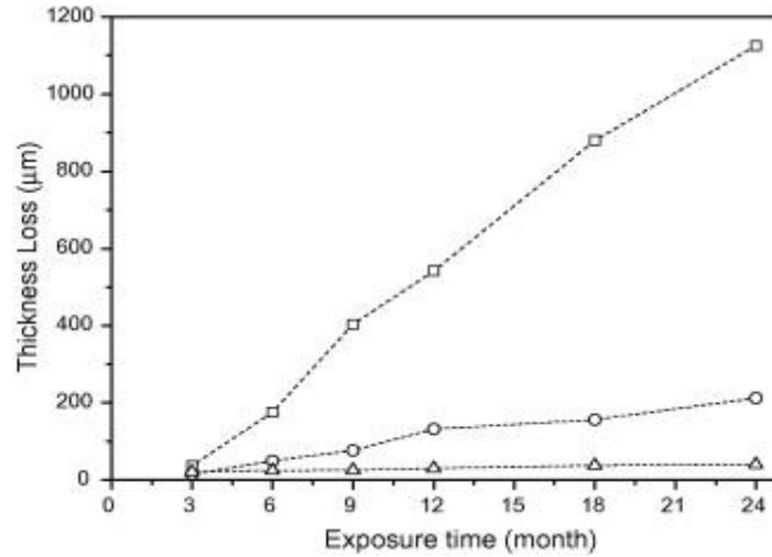
Figure 2. Thickness loss of carbon steel in the different environment as a function of exposure time, □: samples exposed at 95m station far from the sea line, Δ: samples exposed at 375m station far from the sea line, ○: samples exposed at industrial environment [8]
