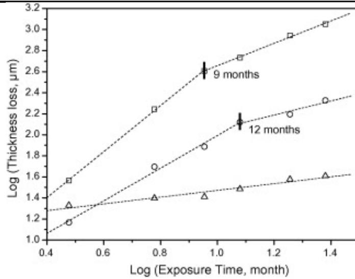
Figure 3. Bilogarithmic plots of data points from Figure 2. □: samples exposed at 95m station far from the sea line; Δ: samples exposed at 375m station far from the sea line; ○: samples exposed at industrial environment [8]
