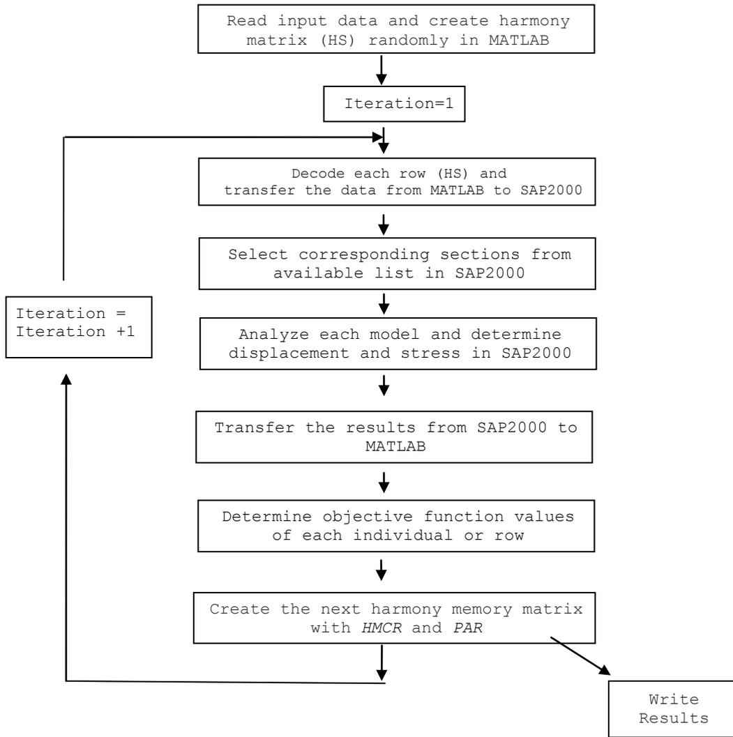
Figure 1. Flowchart for the optimum design procedures
