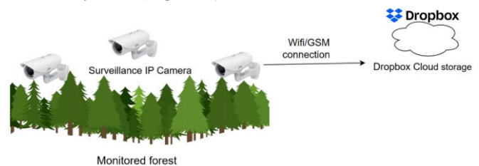
Figure 7. Illustration of image transmission from IP camera to Dropbox
