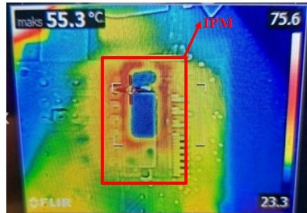
Fig 16. IPM temperature graph at tested switching
