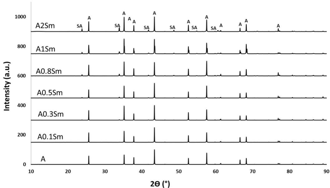
**Figure 1.** The XRD diffraction patterns of the Al<sub>2</sub>O<sub>3</sub>-Sm<sub>2</sub>O<sub>3</sub> ceramics prepared with different Sm<sub>2</sub>O<sub>3</sub> volume ratios.
