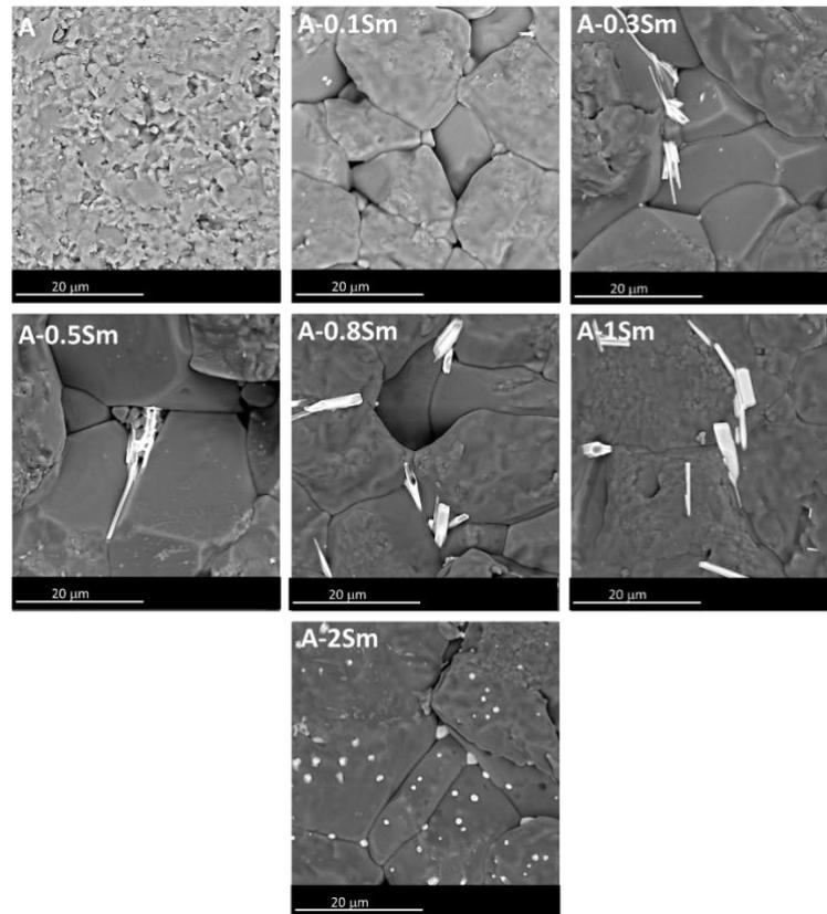
**Figure 2.** SEM images of the thermally etched Al<sub>2</sub>O<sub>3</sub>-Sm<sub>2</sub>O<sub>3</sub> ceramics sintered at 1550°C.
