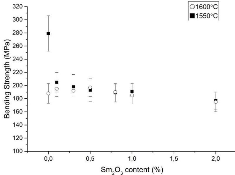
**Figure 5.** The bending strength of Al<sub>2</sub>O<sub>3</sub>-Sm<sub>2</sub>O<sub>3</sub> ceramics as a function of Sm<sub>2</sub>O<sub>3</sub> volume content for the sintering temperature.
