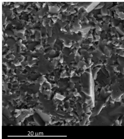
**Figure 6.** SEM image of the fracture surface of the Al<sub>2</sub>O<sub>3</sub> sintered at 1550°C.
