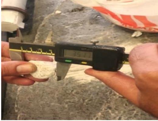
**Figure 5.** Dimensional properties of the mucus materials taken as samples
