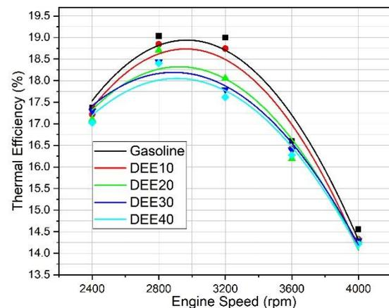
Fig. 5. Changes of thermal efficiency
