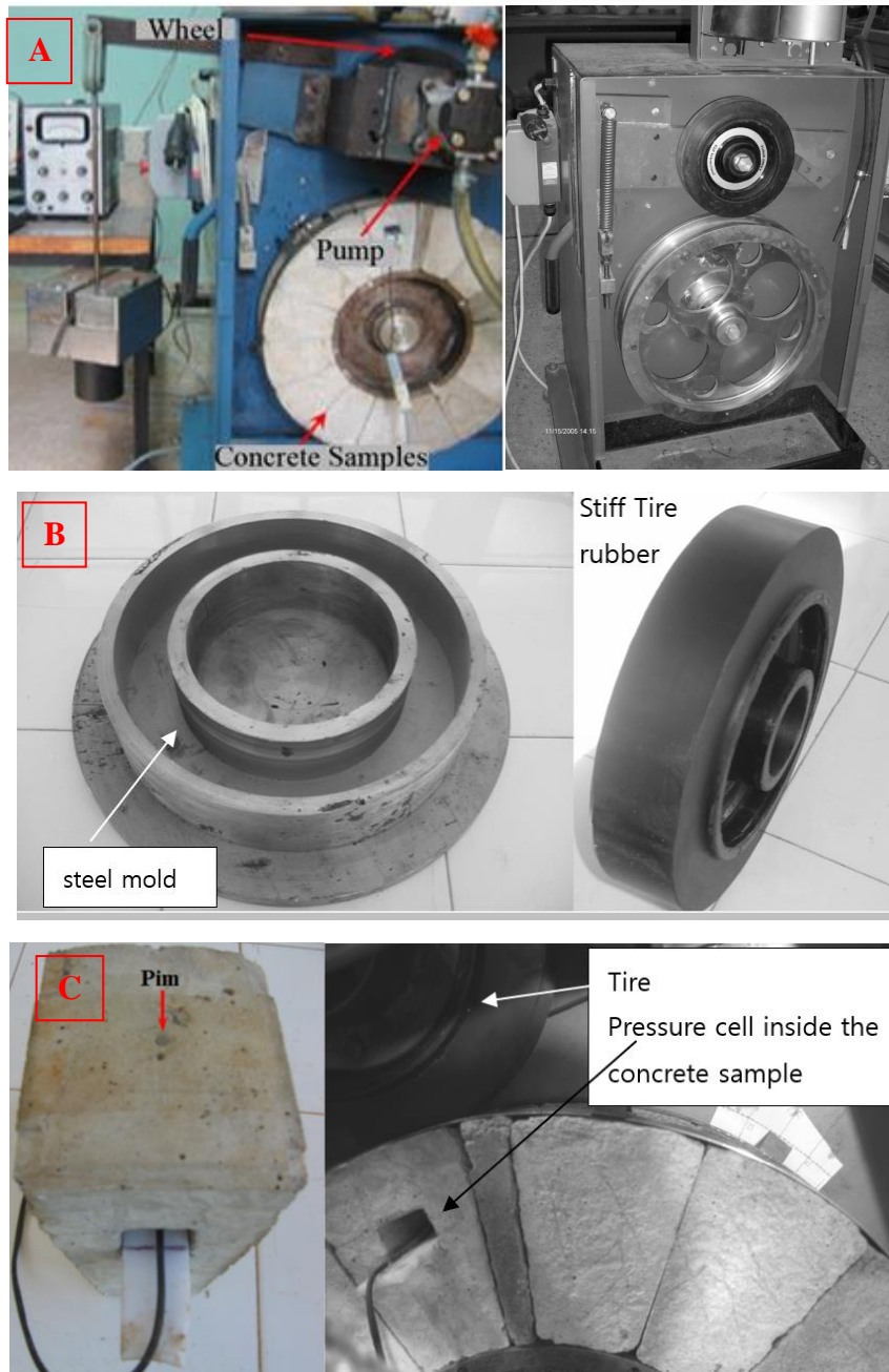
Figure 1. Test setup (a) accelerated polishing test machine setup, (b) mold and small tire (c) vertical pressure cell inside the sample
