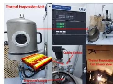
**Figure 1.** Detailed View of the Device of the Thermal Evaporation System
