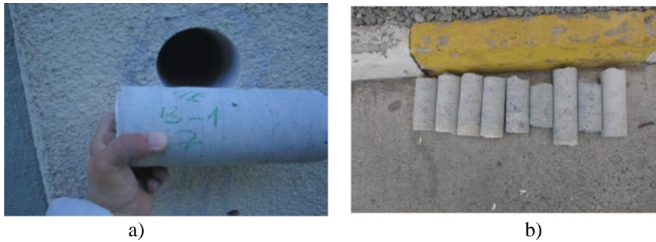
Figure 4. a) b) Concrete core sampling
