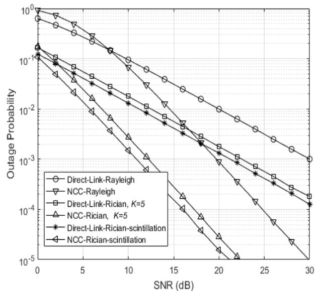
Figure 2. Outage Probability to SNR graphs in direct links and NCC links
