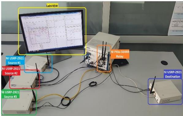
**Figure 3.** Testbed for the proposed NCC system model with SDR nodes
