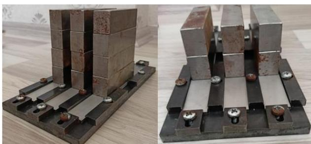
Figure 5. Applying pressure to the adhesive layer using weight
