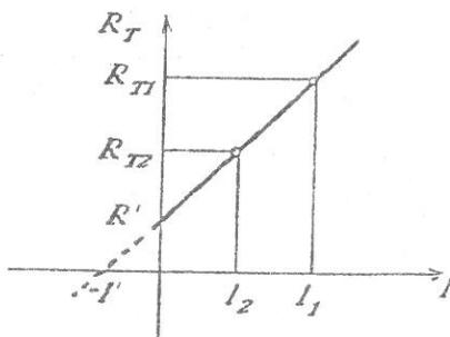
Fig.4. Total resistance as a function of  $l$ .
