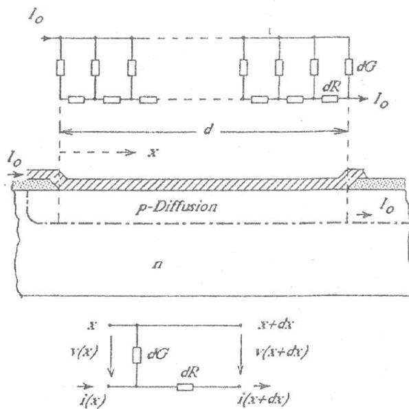
Fig.3. Transmission line model for the planar contact [1].
