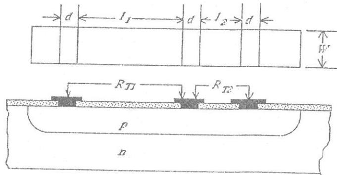
Fig.2. The three-terminal resistor structure.
