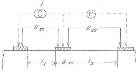
Fig.5. Experimental setup for obtaining total resistance and contact end resistance values [5].
