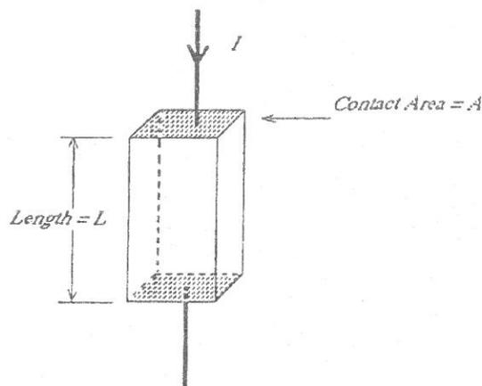
Fig.1. The two-terminal resistor structure.
