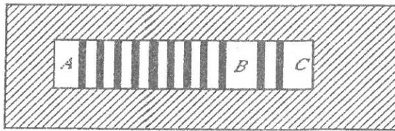
Fig.7. Test pattern for contact resistivity measurement. Dark areas represent bare semiconductor surfaces; cross-hatched area represents a region etched below the p-n junction for isolation [9].
