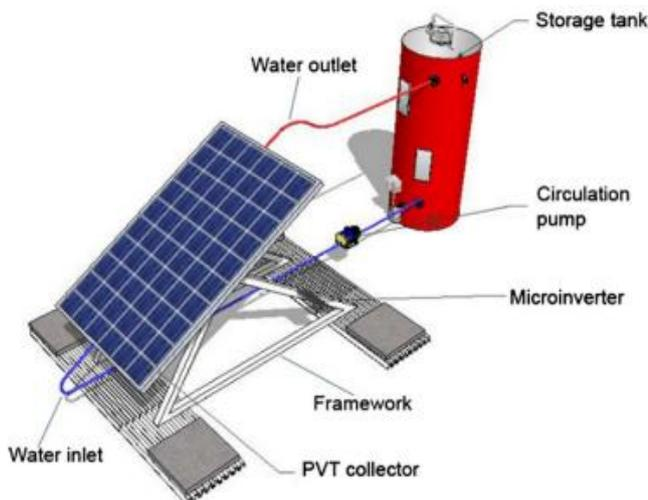
Figure 3 Water cooling [20]
