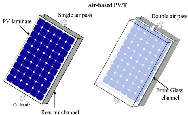
Figure 2 Air based PV/T (single and double) [15]
