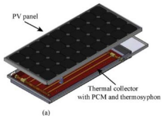
Figure 5 Cooling with PCM [27]
