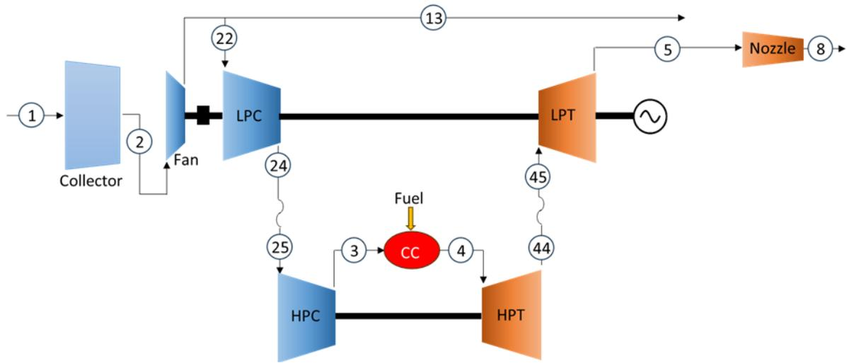
Thermodynamic schematic of the modelled engine
