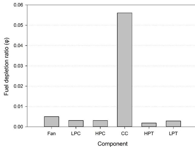
**Figure 8.** Fuel depletion ratios of the components
