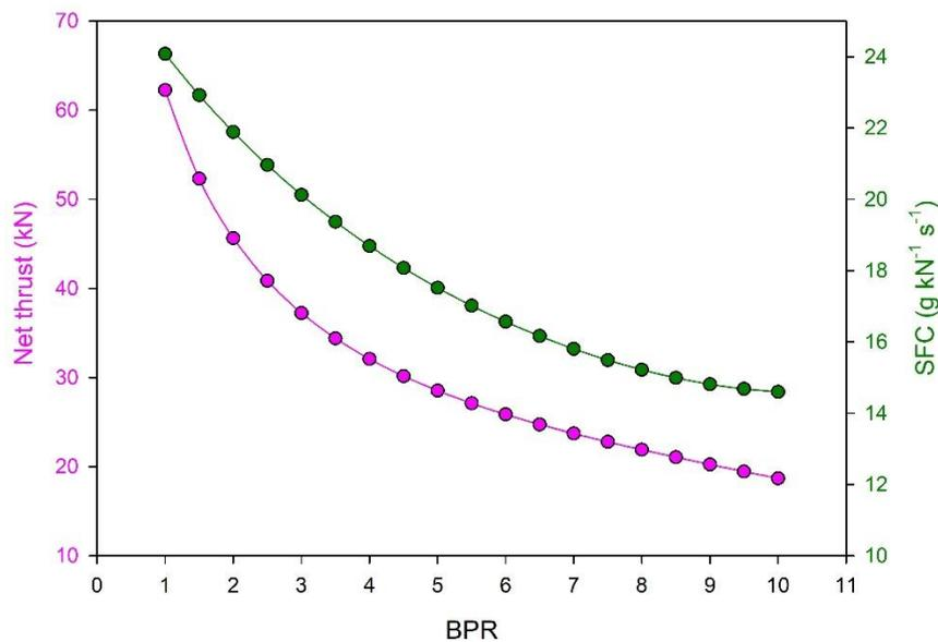
Figure 9. Net thrust and SFC variation relative to BPR
