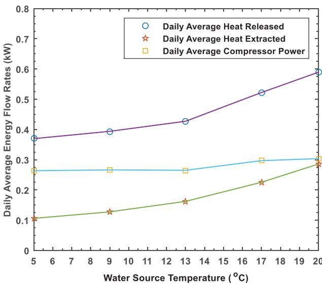
**Figure 5.** Effect of water source temperature on the daily average energy flow rates.
