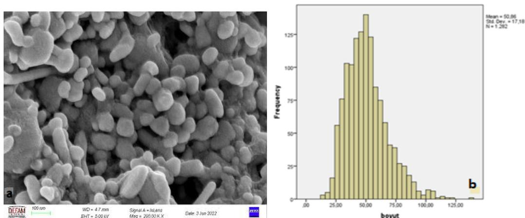
**Figure 8- SEM results of nanoparticles obtained from the extract at 20 °C: (a) 200.00 K X, (b) histogram graph of nanoparticle size**
