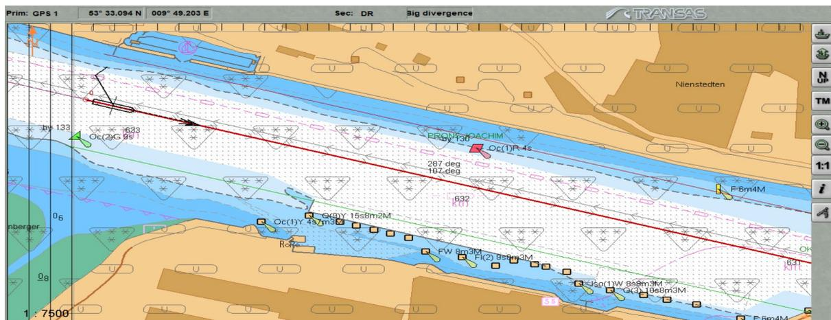
Figure 4. CATZOC display on ECDIS screen (Transas, 2020)
