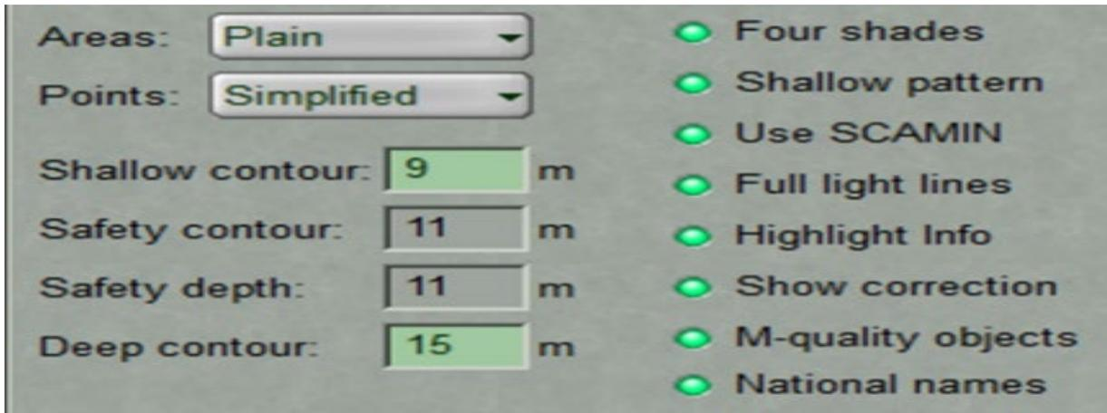
Figure 8. Safety parameters entered into ECDIS
