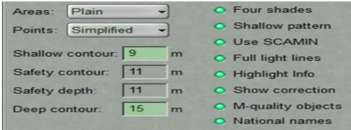
Figure 8. Safety parameters entered into ECDIS
