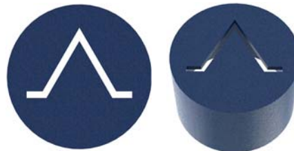
Figure 5. Orifice shape of single wave
