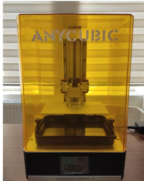
**Figure 2.** Anycubic Photon Mono X 3D printer.
