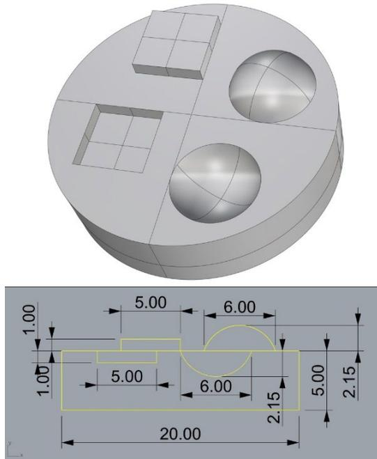
**Figure 1.** 3D view and technical drawing of the printed parts.
