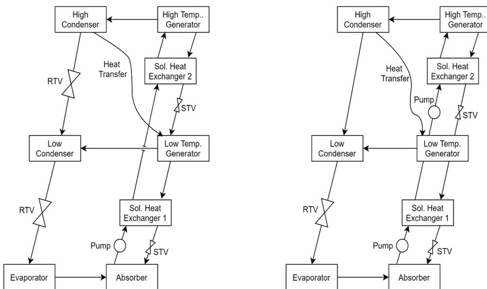
**Figure 4.** Schematic of double effect ARS (a) Series Flow Mode (b) Parallel Flow Mode.
