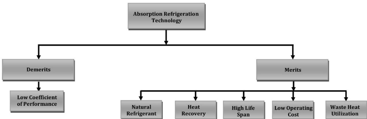
Figure 2. Merits and demerits of absorption refrigeration technology.
