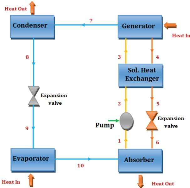
Figure 1. Schematic of SE-ARS.
