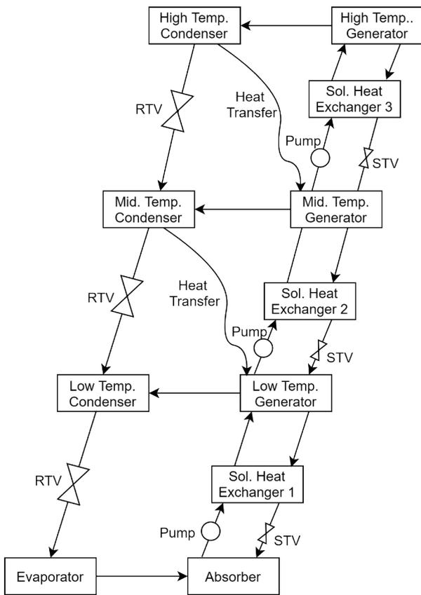
**Figure 5.** Schematic of triple effect ARS (b) Parallel Flow Mode.
