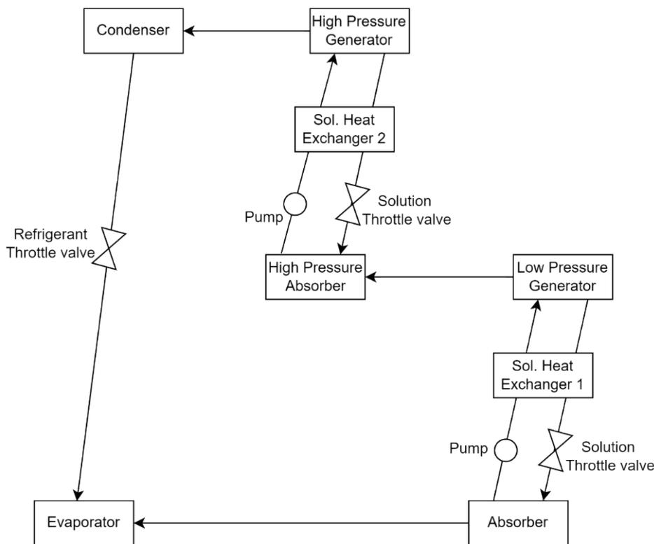
Figure 3. Schematic of half effect ARS.
