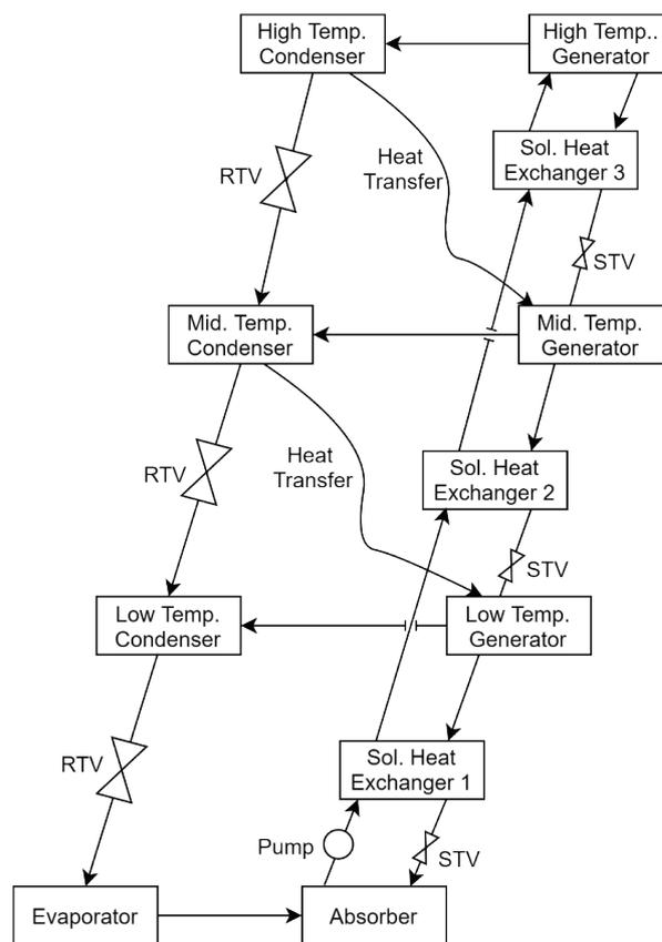
**Figure 5.** Schematic of triple effect ARS (a) Series Flow Mode.
