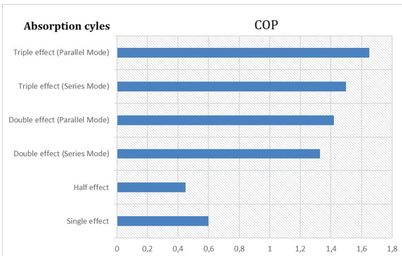
**Figure 6.** COP comparison for different ARSs.
