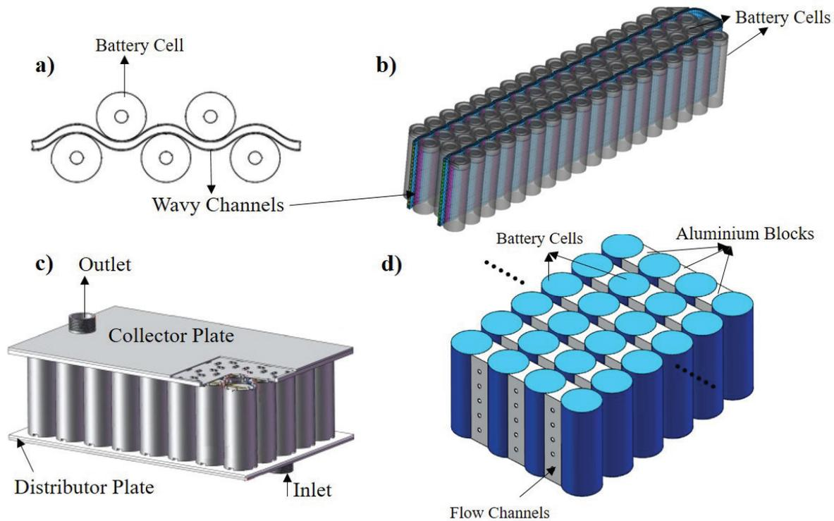
**Figure 6.** (a) The schematic of wavy channel [126] (b) The schematic of the battery pack using wavy channels [128], (c) the schematic of LCCs including 40 battery cells [130], (d) the schematic of battery pack using cooling blocks with liquid channels [131].
