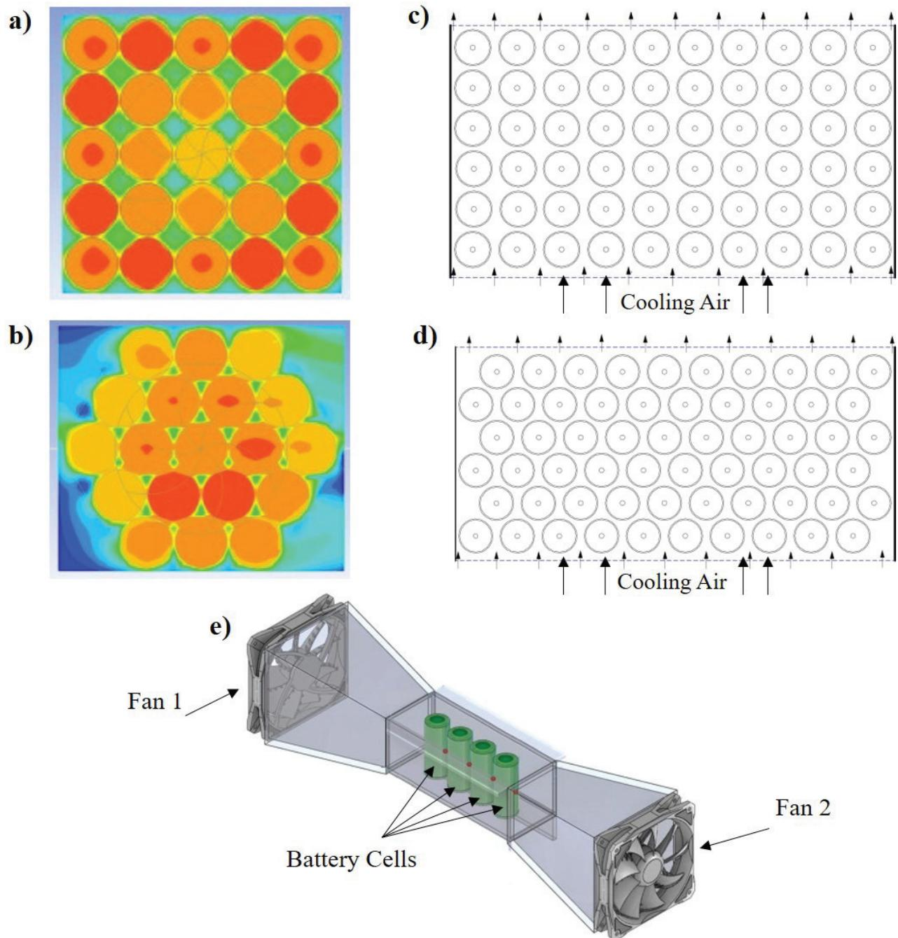
**Figure 5.** (a-b) The cubic and hexagonal structure when the fan is positioned at the top of module [116], c-d) the aligned and staggered cell layouts [117], e) the battery module cooling with the active control using reciprocating air flow [118].
