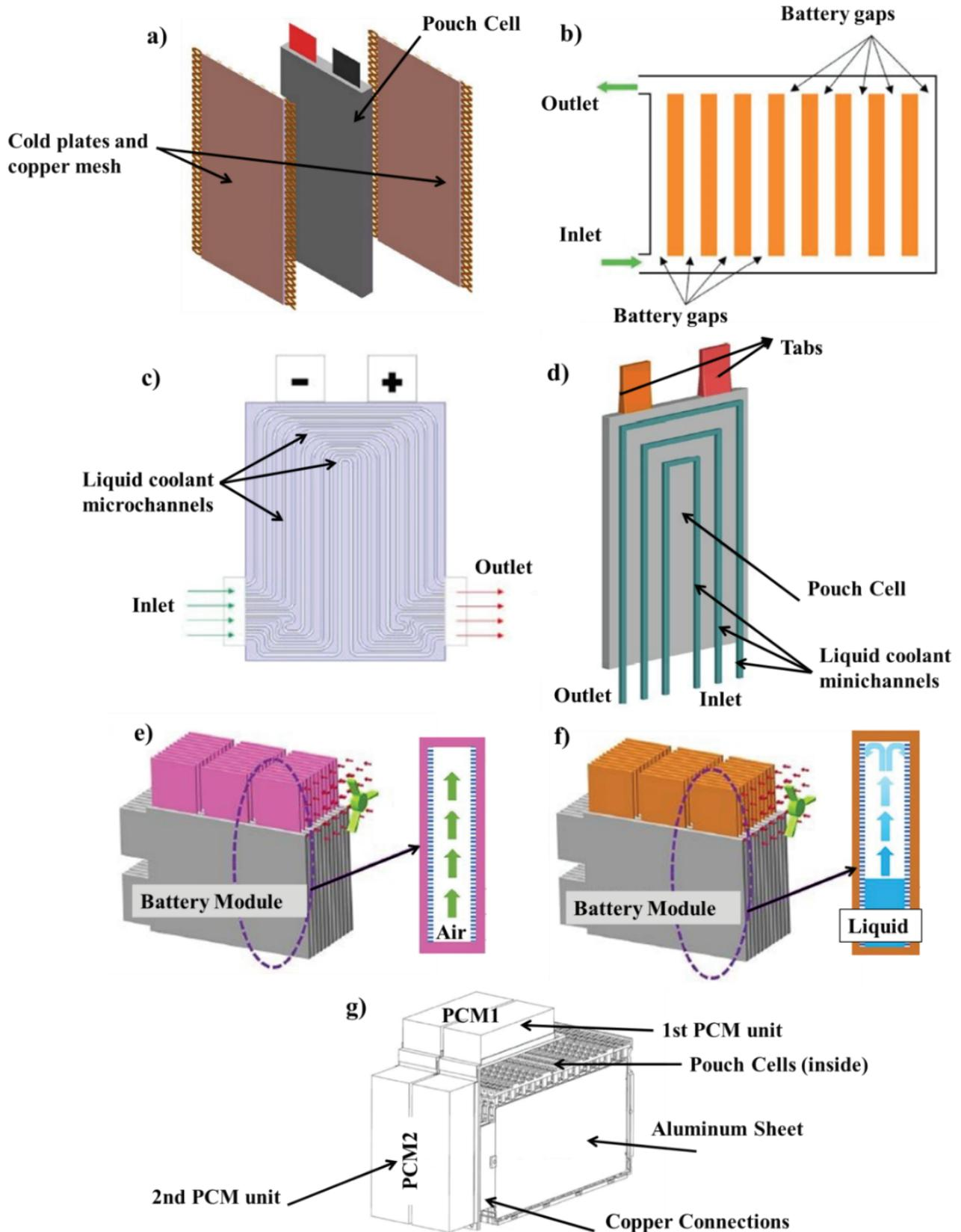
**Figure 4.** BTMS strategies for pouch type battery cell and pack, a-b) air-cooling [93, 94], c-d) liquid cooling [97, 98], e-f) heat pipe cooling [102] and g) PCM cooling [106].
