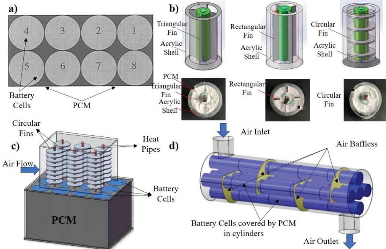
**Figure 7.** (a) The proposed PCM-based cooling EV module [141] (b) Three different fin cases and corresponding experimental images [148], (c) PCM/finned-HP integrated thermal management module [149], (d) the PCM integrated shell and tube battery pack [150].
