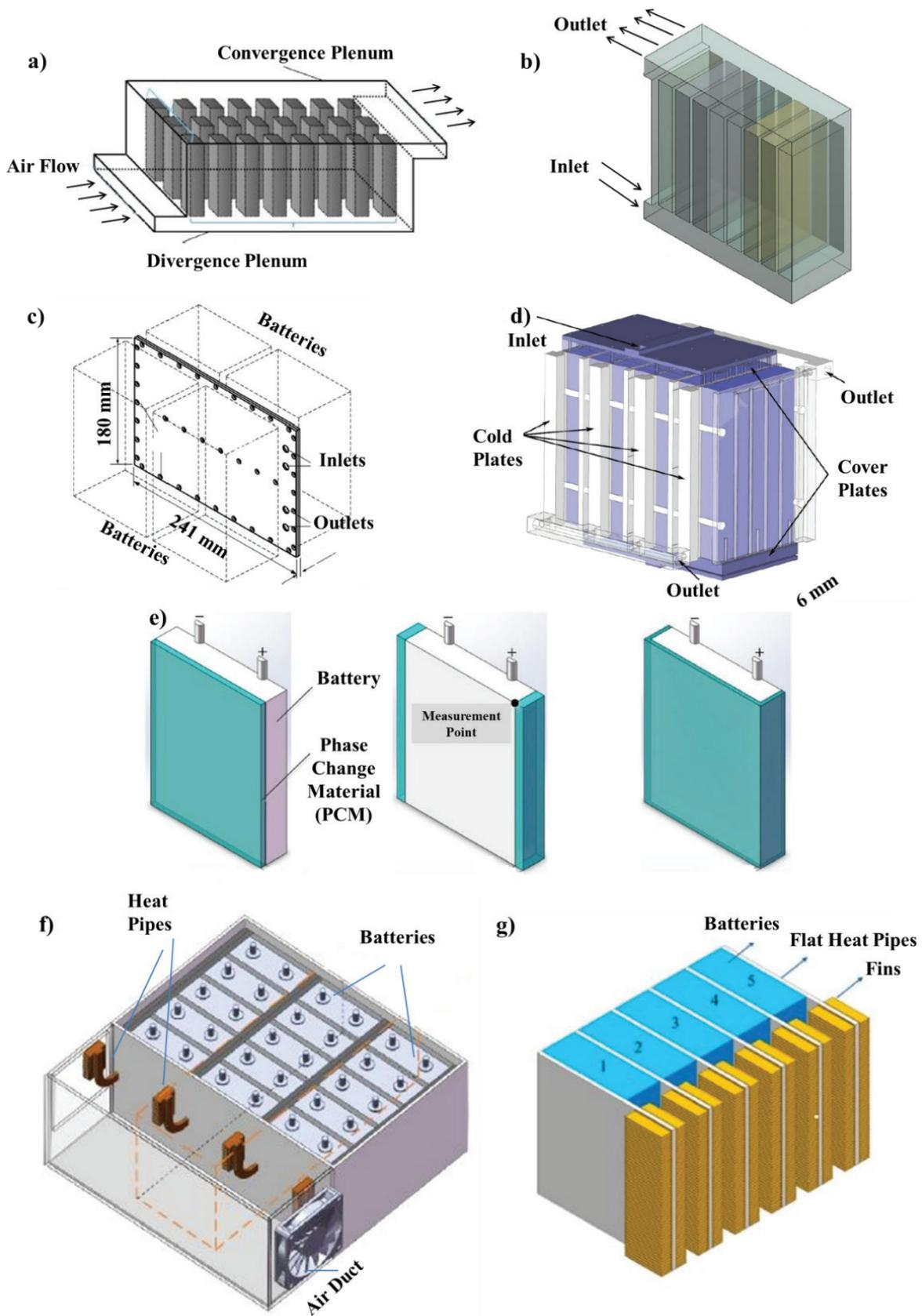
**Figure 3.** BTMS strategies for prismatic battery cell and pack, a-b) air-cooling [58, 59], c-d) liquid cooling [64, 67], e) PCM cooling [72], f) PCM-heat pipe integrated cooling [73], and g) heat pipe cooling [74].
