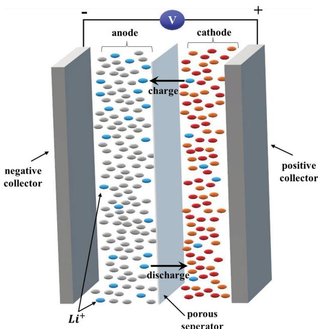
Figure 1. Main sublayers of a Li-ion battery cell.
