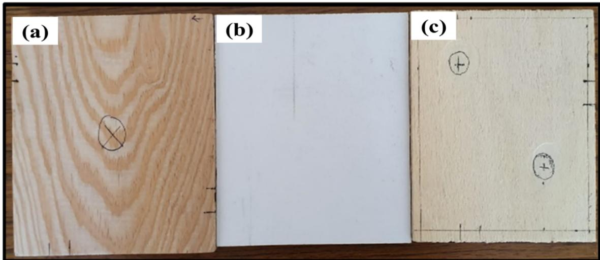
**Figure 1.** Images of the wooden materials used in this research: (a) pine, (b) MDF laminate, and (c) poplar
