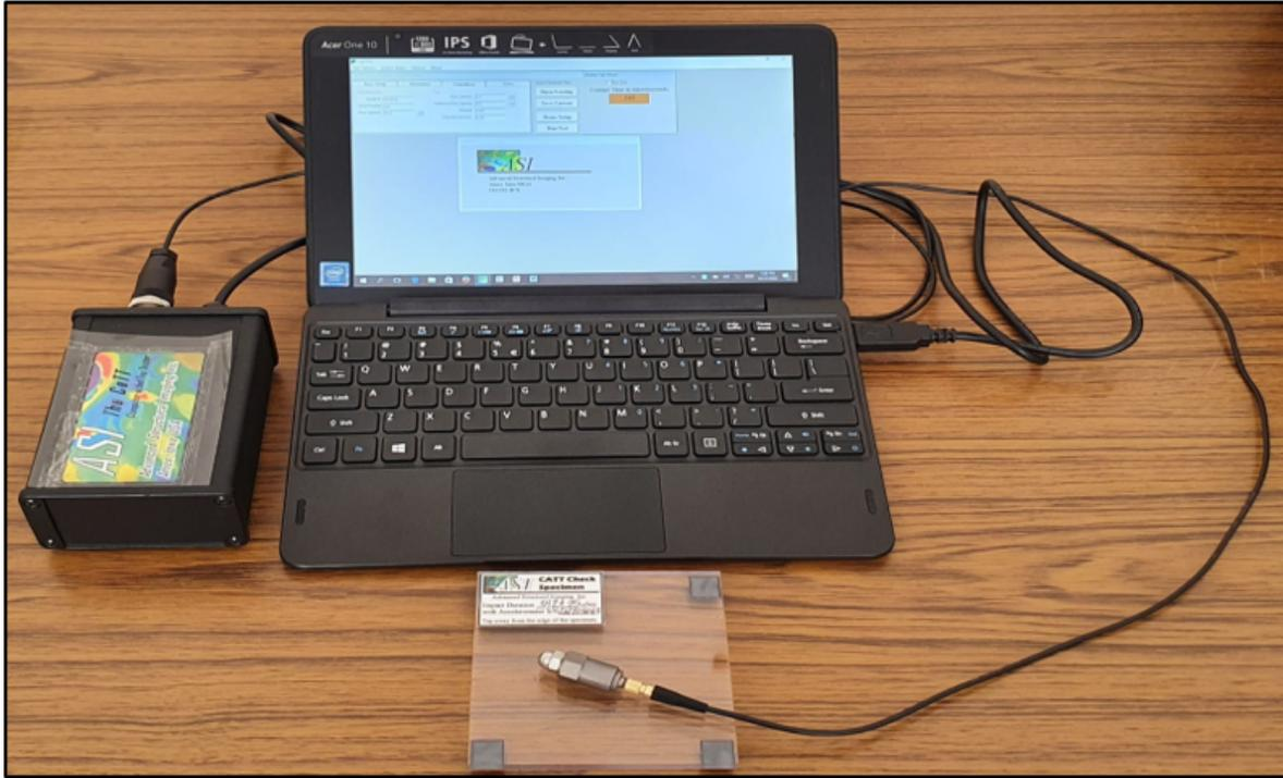
**Figure 2.** The computer-aided tap tester system used in this research
