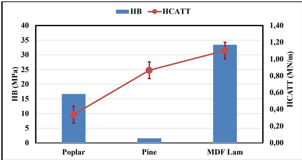
Figure 3. Brinell hardness values (HB) and computer-aided tap test hardness values (HCATT) for some wooden materials.
