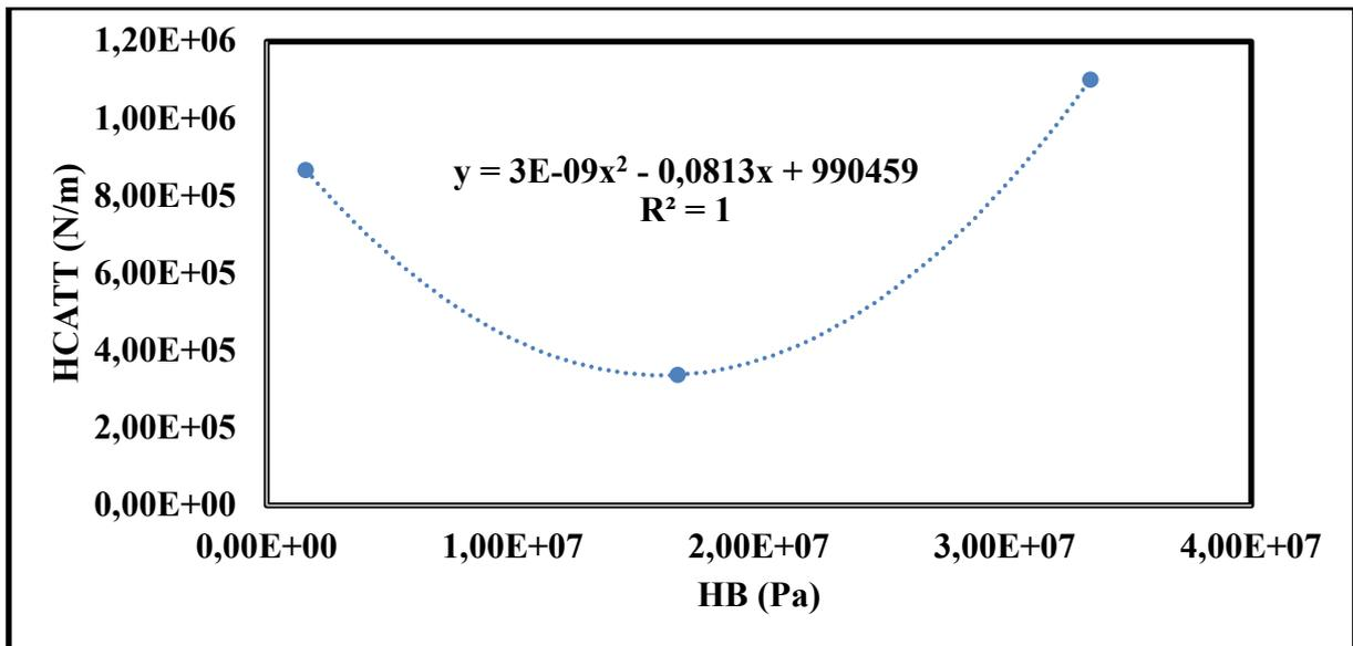
Figure 4. Relationship between Brinell hardness values (HB) and computer-aided tap test hardness values (HCATT) for some wooden materials.
