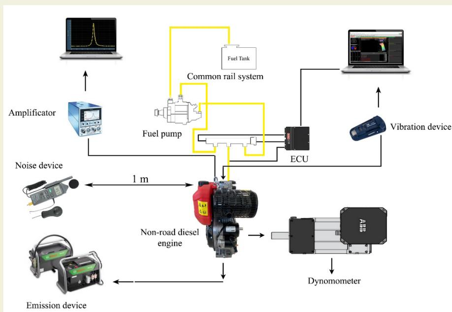
**Figure 1.** The schematic representation of the engine setup and the measurement devices used in the tests.
