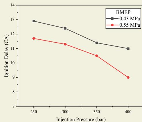
**Figure 3.** Variation of ID for non-road single-cylinder diesel engine at varying DIP.
