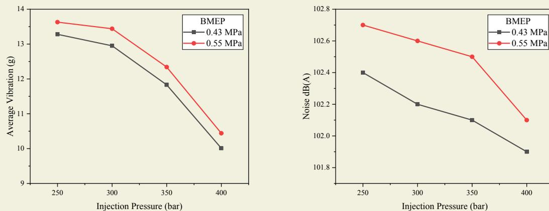
**Figure 7.** Variation of vibration and noise emissions for non-road single-cylinder diesel engine at varying DIP.
