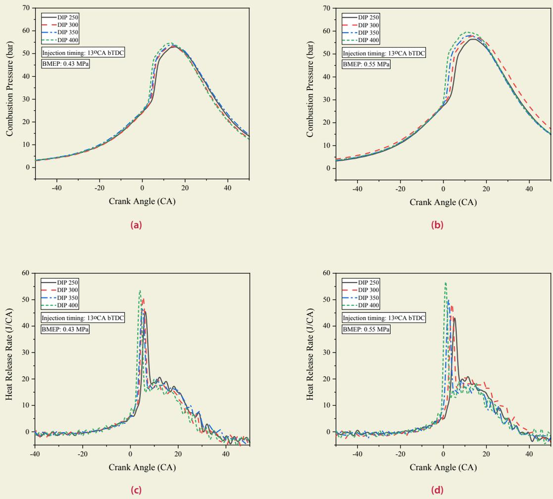
**Figure 2.** Variation of combustion pressure and HRR for non-road single-cylinder diesel engine at varying DIP.
