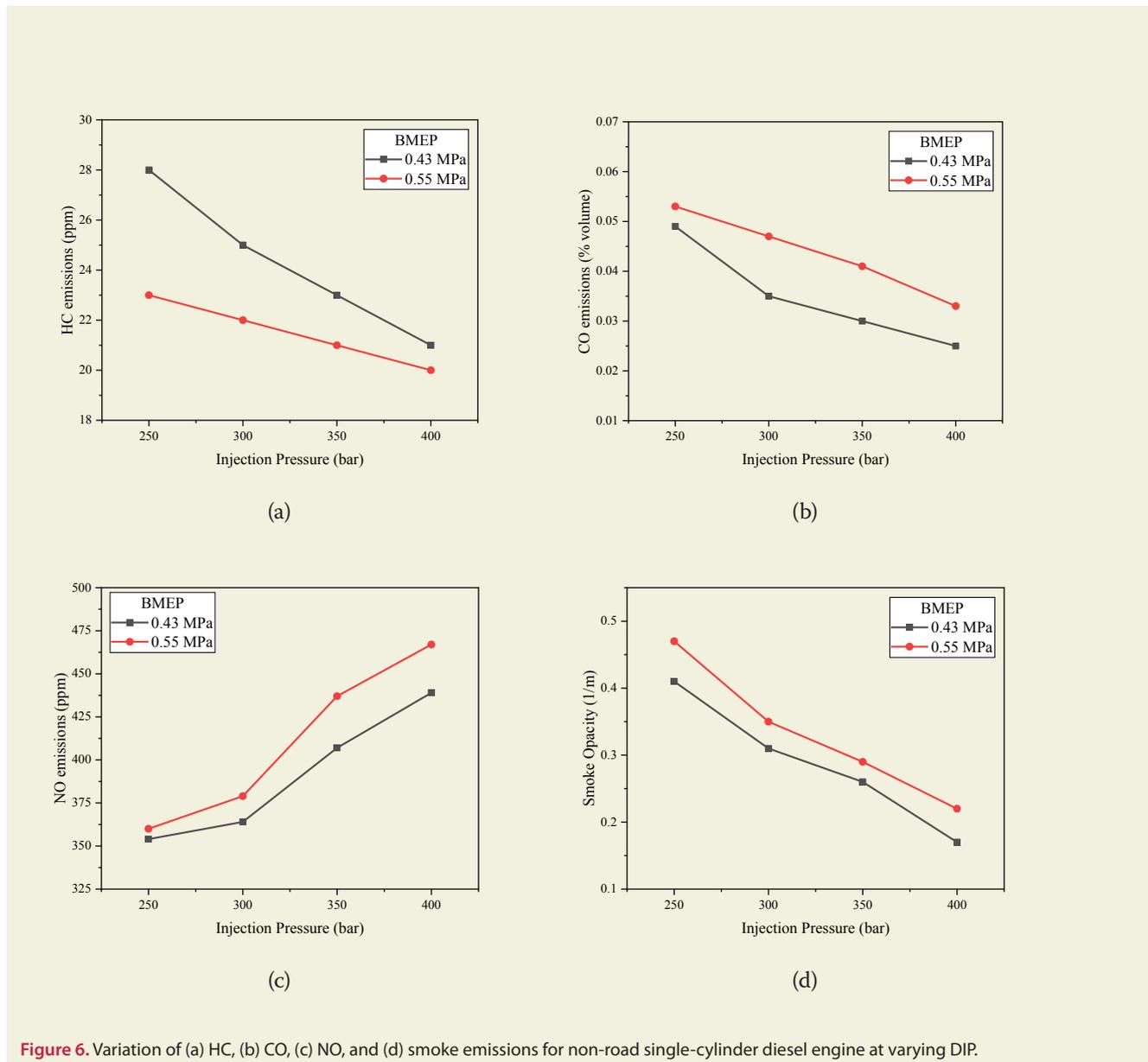
Figure 6. Variation of (a) HC, (b) CO, (c) NO, and (d) smoke emissions for non-road single-cylinder diesel engine at varying DIP.
