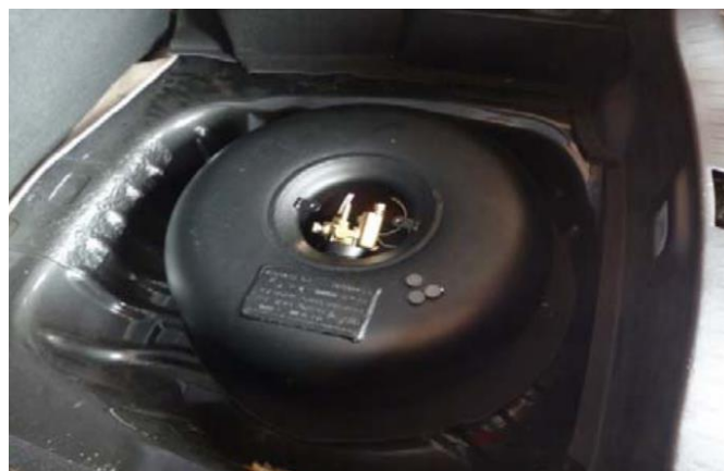
Fig. 1. An LPG tank that fits in the spare tire location (18)
