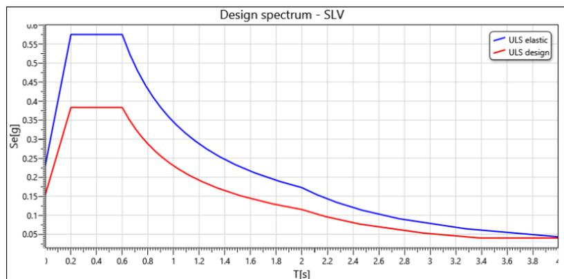
Figure 8. Design spectrum according to Eurocode
