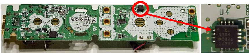
Fig. 6. The ADXL330 Accelerometer In "Wii Remote"
