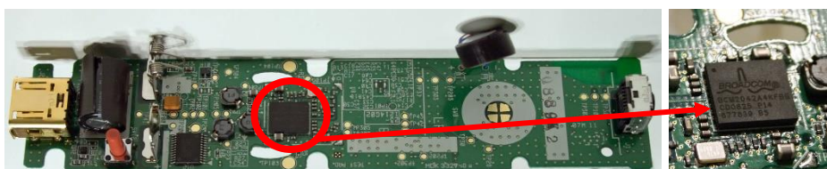
Fig. 7. "Wii Remote" With The BCM2042 Microcontroller
