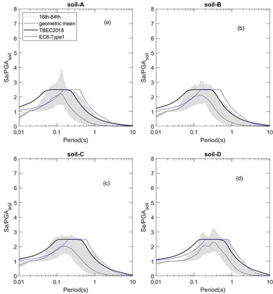
**Figure 7.** Normalised real spectral accelerations with their geometric mean and 16th-84th percentiles along with the design response spectra guided by TBEC 2018 and EC8
