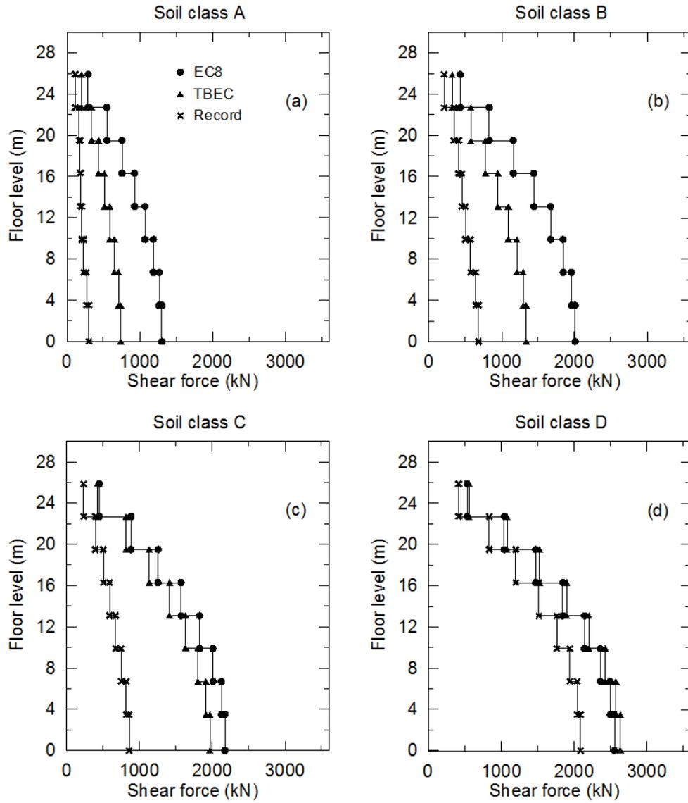
**Figure 11.** Shear force distributions, along the 8 storey building model, from the building analyses conducted by considering the EC8, TBEC design response spectra and actual spectral response curves at different soil classes
