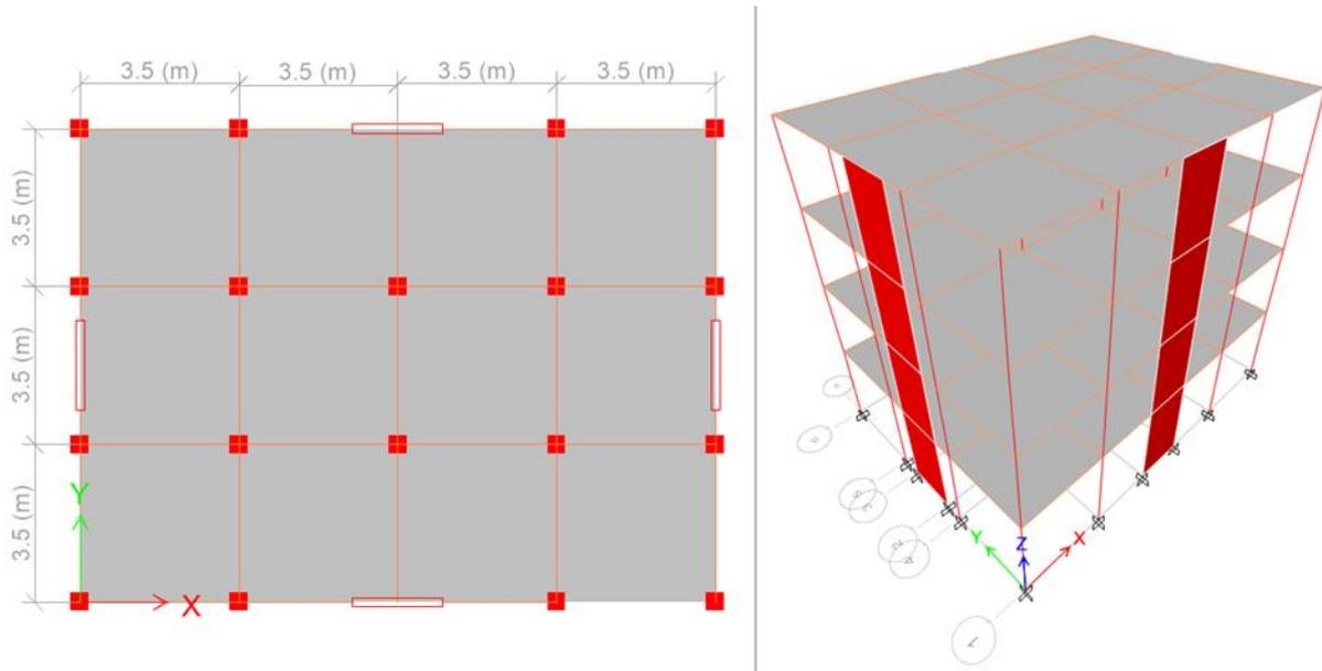
**Figure 8.** The plan and three-dimensional views of the 4 storey building model
