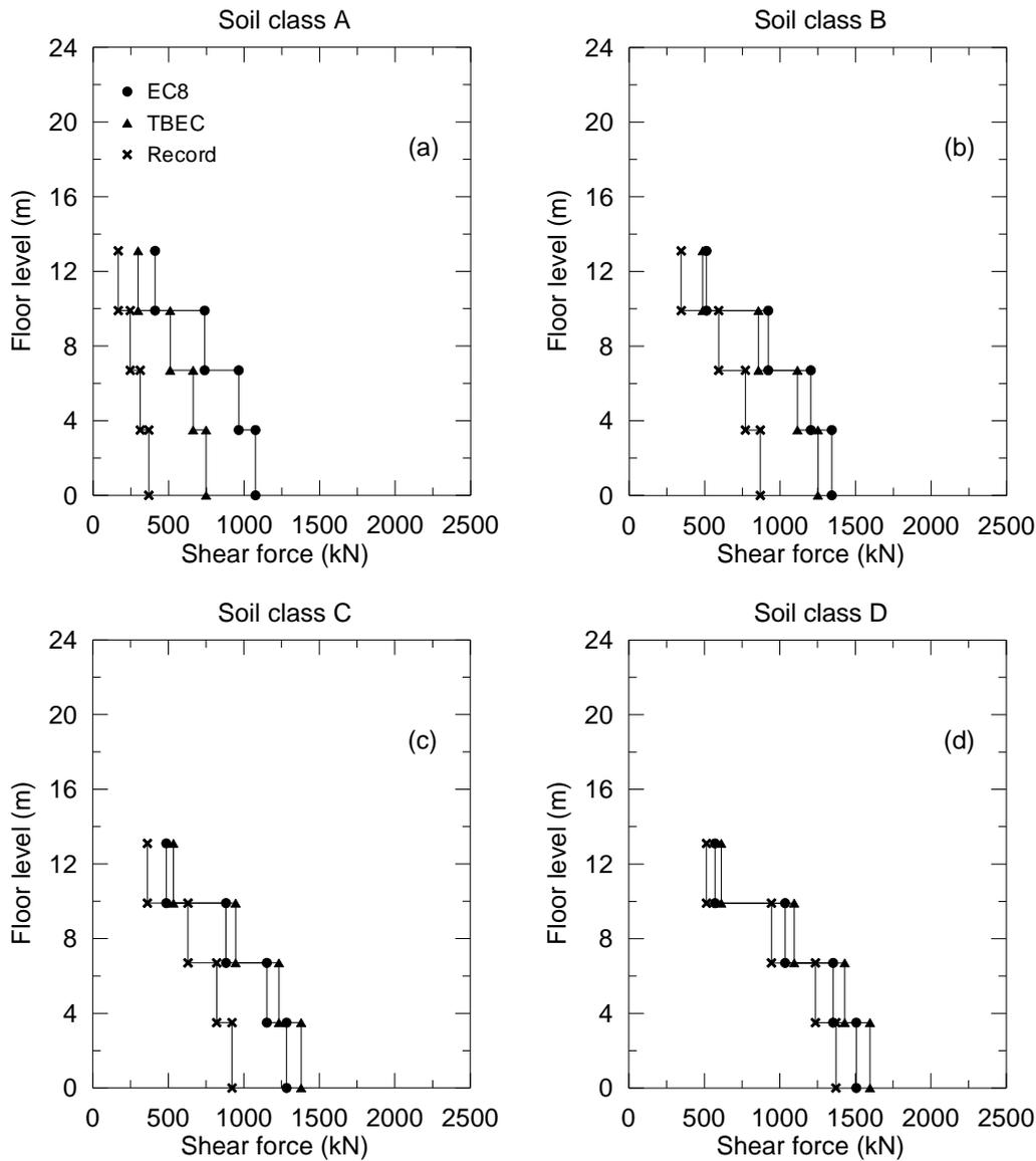
**Figure 10.** Shear force distributions, along the 4 storey building model, from the building analyses conducted by considering the EC8, TBEC design response spectra and actual spectral response curves at different soil classes
