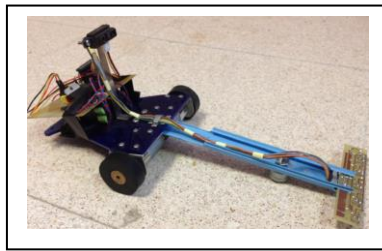
Figure 4. The Line Follower Robot (CIURunner)
