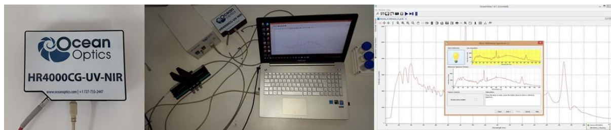
Figure 2. From Left To Right: Spectrometer, Whole Measurement System And Software.
