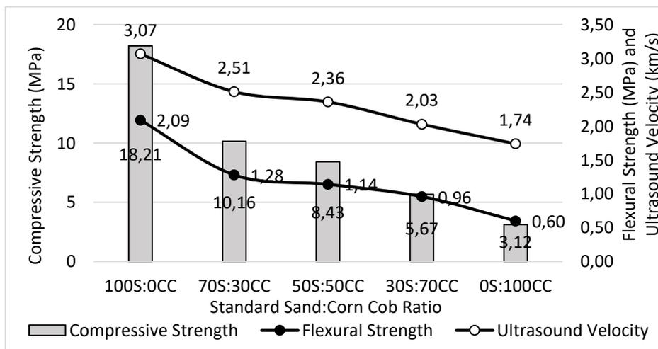
Figure 11. The effect of the S:CC ratio on ultrasound velocity, compressive and flexural strength relationship of NP-based geopolymer mortar
