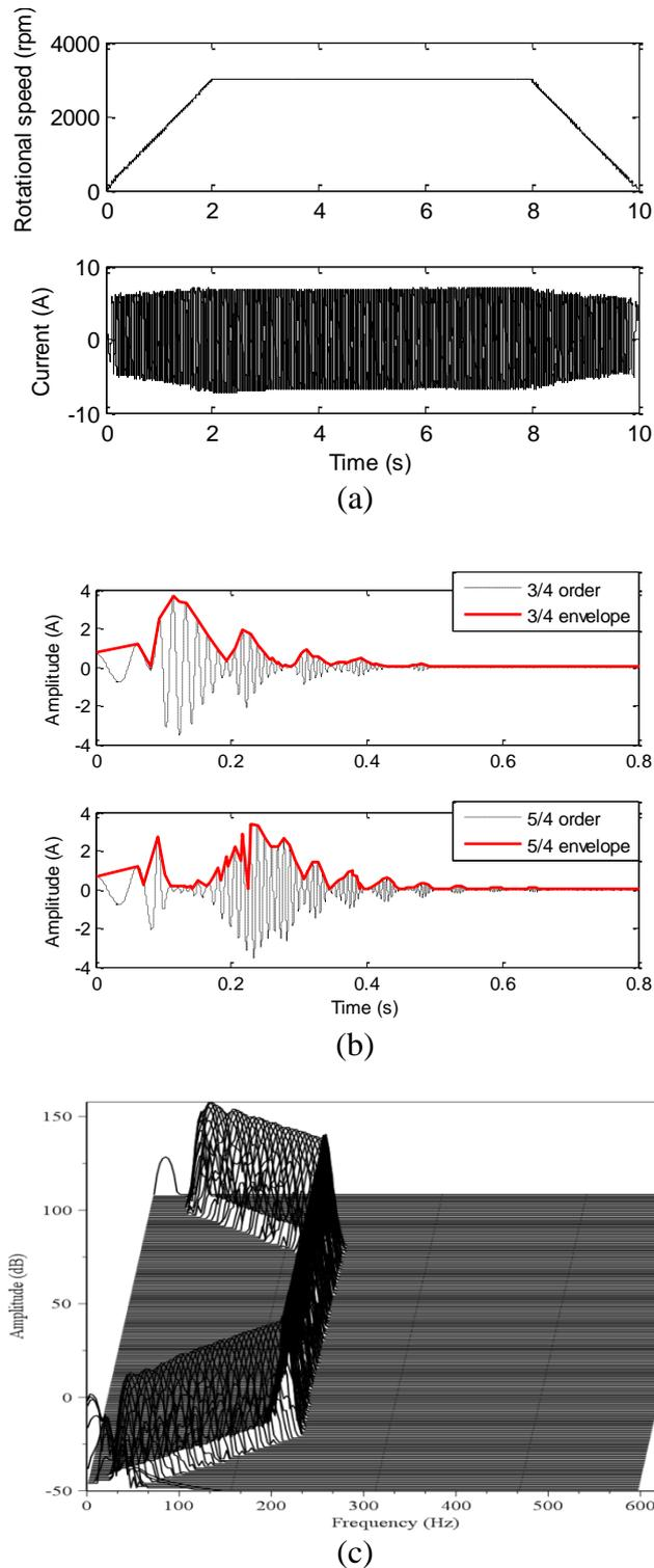
**Figure 2:** GOT results for healthy PMSM with speed profile 0-3000-0 r/min. ( a) Rotational speed and stator current. (b) Tracked 3/4 and 5/4 orders and corresponding envelopes of stator current. (c) Waterfall graph of the tracked orders.
