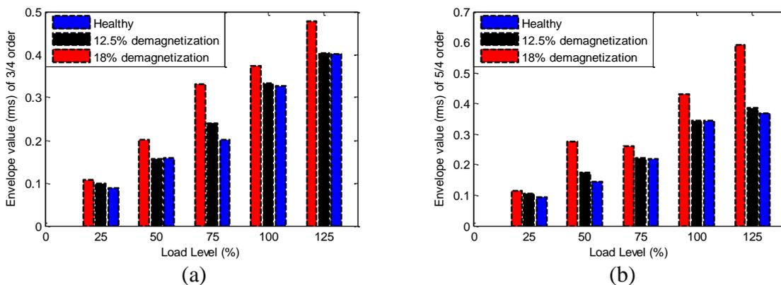
**Figure 4:** Envelope value (rms) of fault characteristic orders for PMSM with partial demagnetization fault under different load levels. (a) Tracked 3/4 order envelope value. (b) Tracked 5/4 order envelope value.
