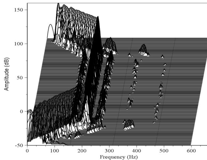
**Figure 3:** Waterfall graph of PMSM under 18% demagnetization fault.
