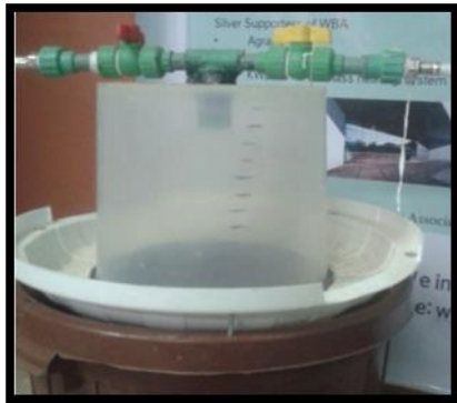
Fig. 4. Gas holder full of biogas.
