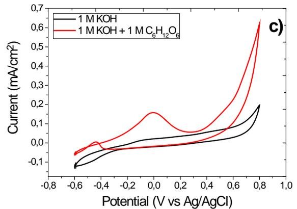
**Figure 3.** CV analyses of **4** and **Pd@4** organic-based catalysts at a scan rate of 50 mV/s a) 1 M KOH, b) 1 M KOH + 1 M C<sub>6</sub>H<sub>12</sub>O<sub>6</sub>, and c) comparison of **Pd@4** organic-based catalyst in 1 M KOH and 1 M KOH + 1 M C<sub>6</sub>H<sub>12</sub>O<sub>6</sub> solutions.
