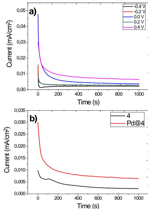
**Figure 4.** CA curves of a) **Pd@4** organic-based catalyst at different potentials and b) comparison of organic-based catalysts at 0.4 V potential in 1 M KOH + 1 M C<sub>6</sub>H<sub>12</sub>O<sub>6</sub> solution.
