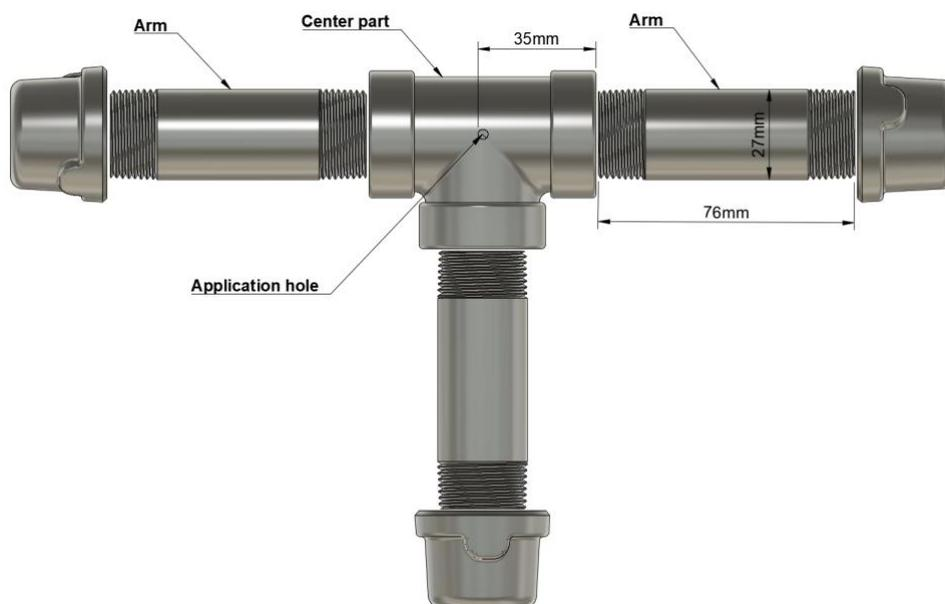
Figure 1. Illustration and dimensions of the olfactometer.
