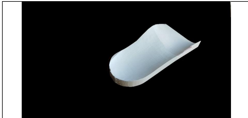
Figure 4. Fresh insole model after printing process
