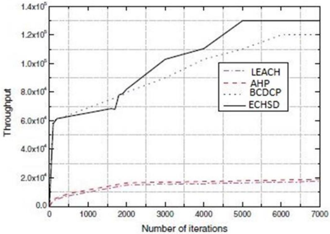
Figure 6. Network throughput when x=0.1.
