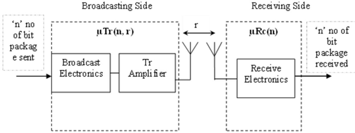
Figure 3. Communication representation for Blue Brain nodes.
