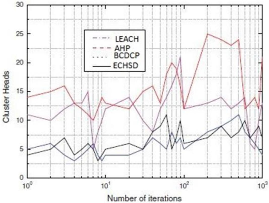
Figure 8. Cluster head amount in particular cycle when  $x = 0.1$ .
